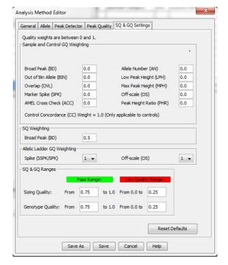
The following screenshots show what parameters should be used when setting up the CODISYfiler\_3500 analysis parameters:
